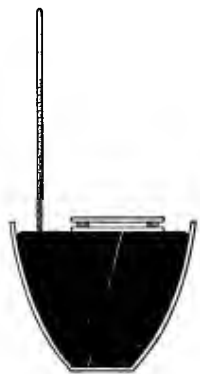
FIG. 151. Crucible Method of Micro-sublimation.
