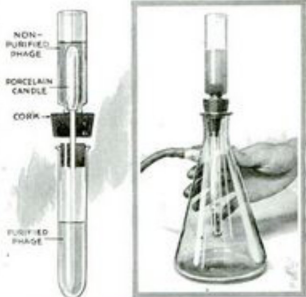
Above, the Berkefeld filter and diagram showing how it works. Through the porcelain candle in bottle's neck the phage is filtered to be sure no germs remain in serum.
