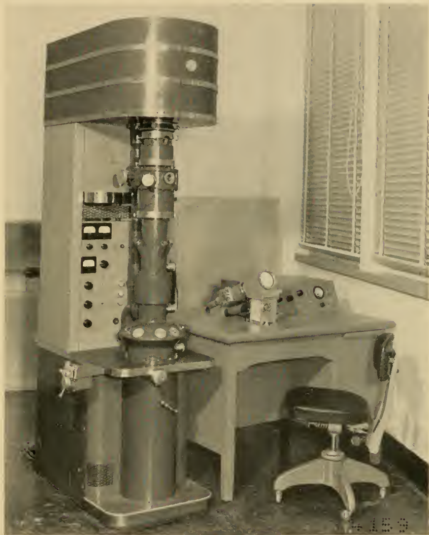
R. C. A. TYPE B ELECTRON MICROSCOPE BESIDE A LABORATORY MODEL OF THE DESK TYPE ELECTRON MICROSCOPE.
